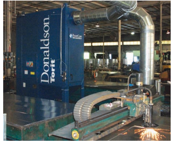
TG on Plasma Cutting 3,400 cfm (5,775 m 3 /h)
