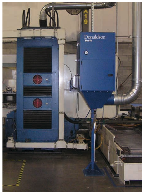
WSO - Horizontal Grinder 850 cfm (1,444 m 3 /h)
