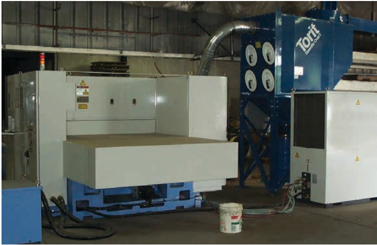
DFO on Laser Cutting 3,100 cfm (5,266 m 3 /h)
