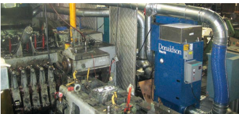
WSO on Cold Forming 1,200 cfm (2,038 m 3 /h)
