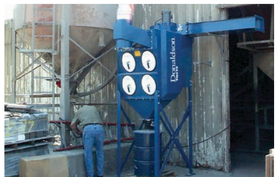
DFO - Concrete Roof Manufacturer 3,000 cfm (5,096 m 3 /h)
