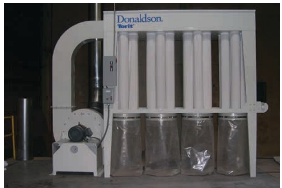
IRD - Wood Shop 5,000 cfm (8,493 m 3 /h)
